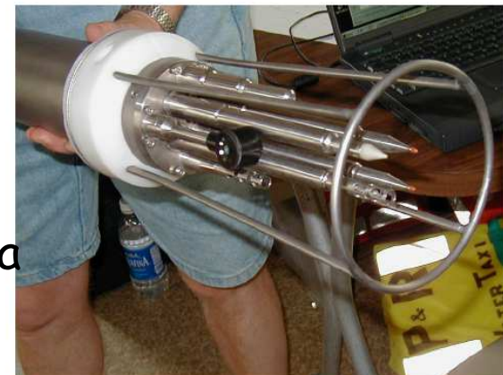
Figure 5: Sensor head of the MSS profiler. The microstructure sensors are standing in front of the other sensors. arrangement guarantees undisturbed measurements of the micro-scale stratification and velocity fluctuations.
