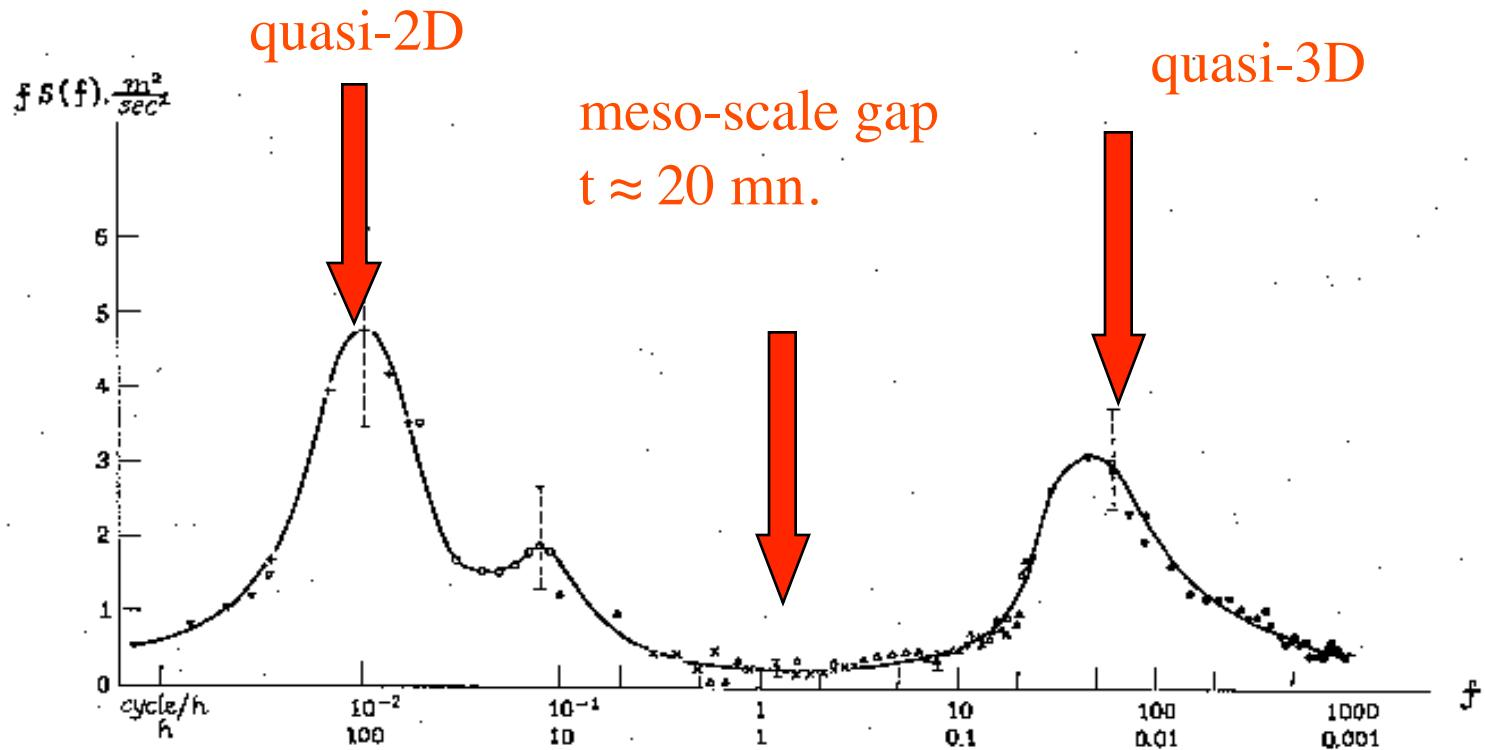
Fig. 3 Spectrum of the horizontal wind velocity. After Van der Hoven.<sup>26</sup> Some experimental points are shown on the graph; see reference 26.
