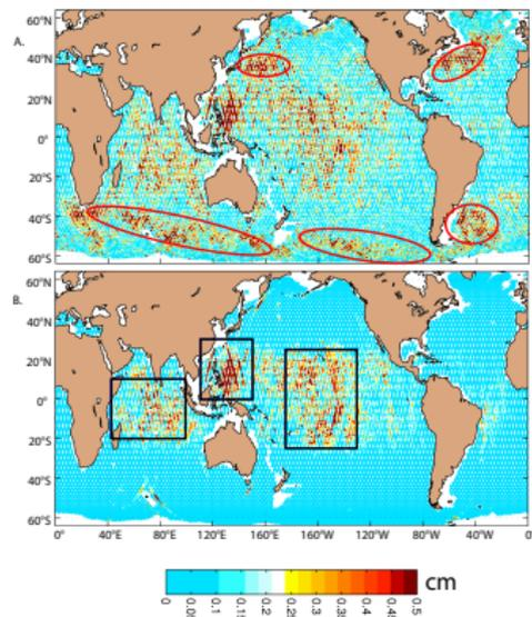
**Figure 8.** The  $K_1$  internal tide amplitude from the (a) altimetric-based and (b) HYCOM tidal analyses. Areas where mesoscale variability contaminates the altimetric-based tidal analysis are identified by the red circles in (a). The three subregions denoted by black boxes in (b) are used to compute the area-averaged amplitudes in Table 3.
