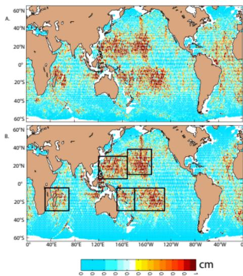
Figure 7. The  $M_2$  internal tide amplitude from the (a) altimetric-based and (b) HYCOM tidal analyses. The five subregions denoted by black boxes in (b) are used to compute the area-averaged amplitudes in Table 2.
