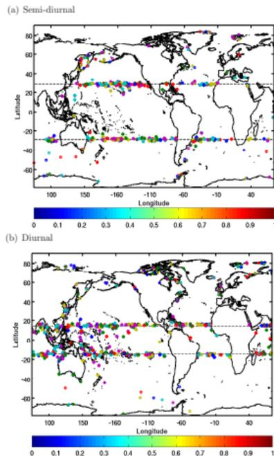
FIG. 4. Global distribution of PSI from the (a) semi-diurnal and (b) diurnal bands. The plots show significant bicoherence values at each grid location from the baroclinic velocities obtained from layer 14 ( $\approx 500$  m depth) of the model. In each case the energy in the subharmonic signals is at least 1% of that of the primary waves.
