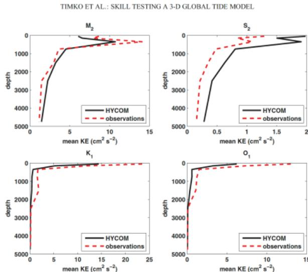
Figure 5. Vertical profiles of the average HYCOM and observed tidal kinetic energy averaged over seven depth bins for the global ocean in deep water (water column depth greater than 1000 m).
